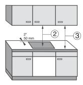
As a general rule there must be a safety distance of at least 30" (760 mm), ②, between the appliance and any flammable objects above it, e.g. cabinetry, venting hood or utensil rail. The minimum distance of combustible surfaces located above and to the side of the cooktop, ③, is 18" (457 mm).
